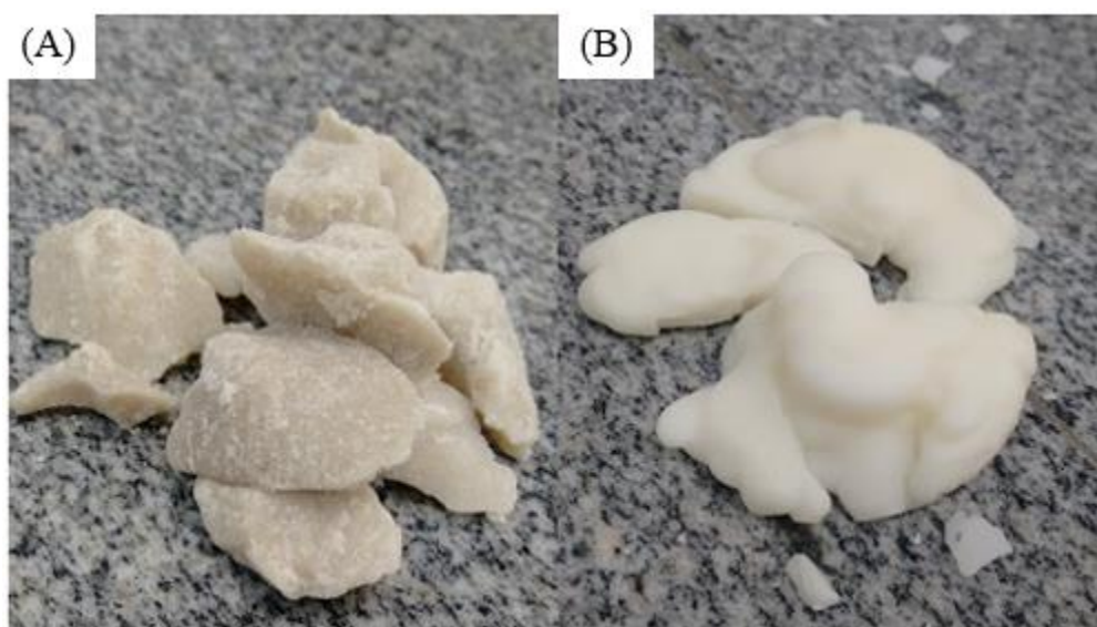
Figure 8 - Images of the crude wax (A) before and (B) after the filtration process.
