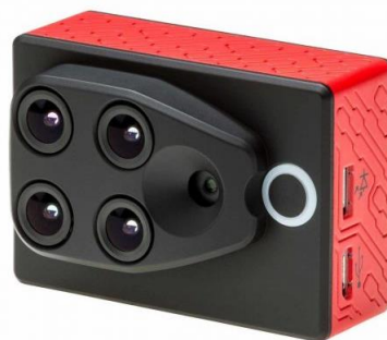
Figura 8 – Sensor multiespectral Parrot Sequoia.
