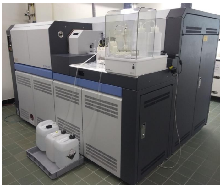
Figure 5. Thermo Scientific Neptune series MC-ICP-MS instrument.
