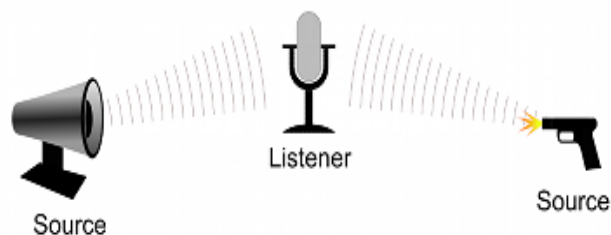
Figura 4.6 – Componentes Áudio Sources e Listener (Unity, 2014)
