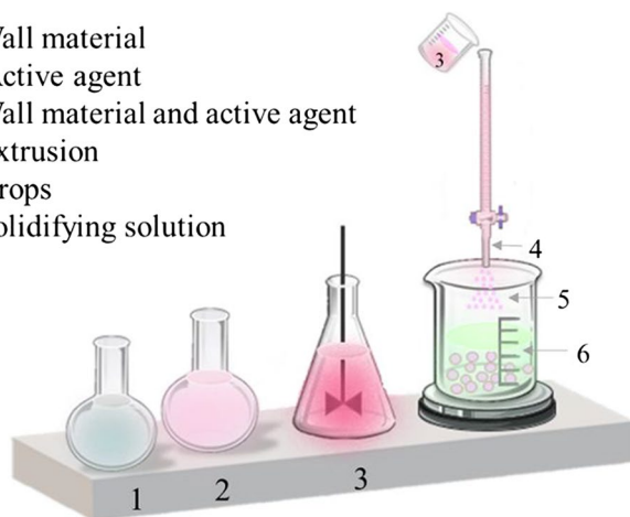
Fig. 3 Scheme of the extrusion method used for phenolic compounds
