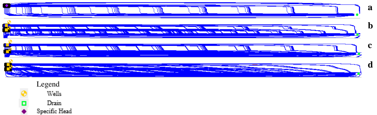
Figure 3.10 – Flow pathlines in the column 12 of the HSSF-CW, considering: a) scenario 01; b) scenario 02; c) scenario 03, and; d) scenario 04
