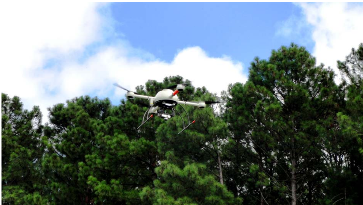
Figura 1 – Microdrone md4-1000 com a câmera Olympus Pen E-P1 .
