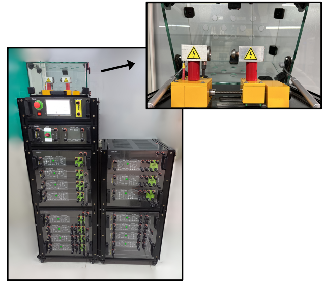
Fig. 6: Arc generator employing the tungsten and nickel-plated copper alloy, according to the IEC 63027 standard.
