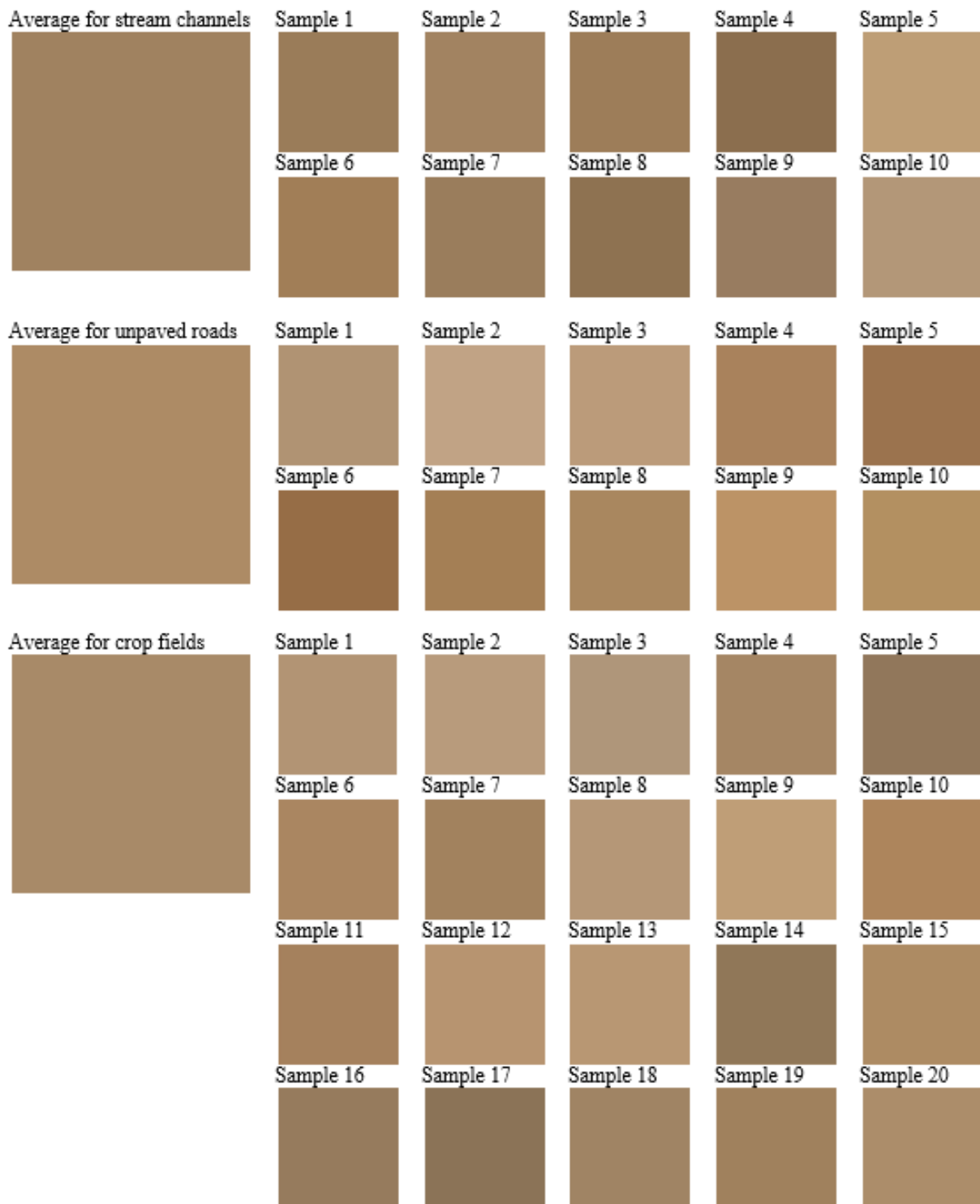
Figure 24 – Colour pictures of the 40 sediment source samples analyzed and the colour picture of the average of stream channel, unpaved road, and crop fields.
