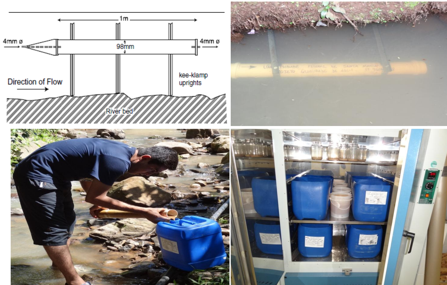
Appendix 1. The specifications of the time integrated suspended sediment sampler used in the study in the Guaporé in the Rio Grande do Sul State, Southern Brazil.
