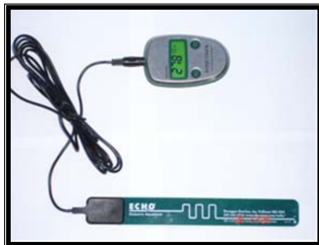
Figura 2.10 - ECH 20 – Dielectric Aquameter (DECAGON DEVICES).
