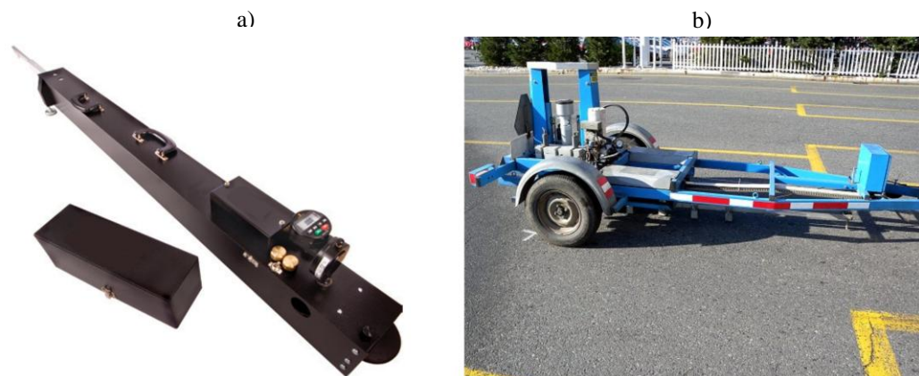
Figura 5 - Viga Benkelman (a) e FWD (b)
