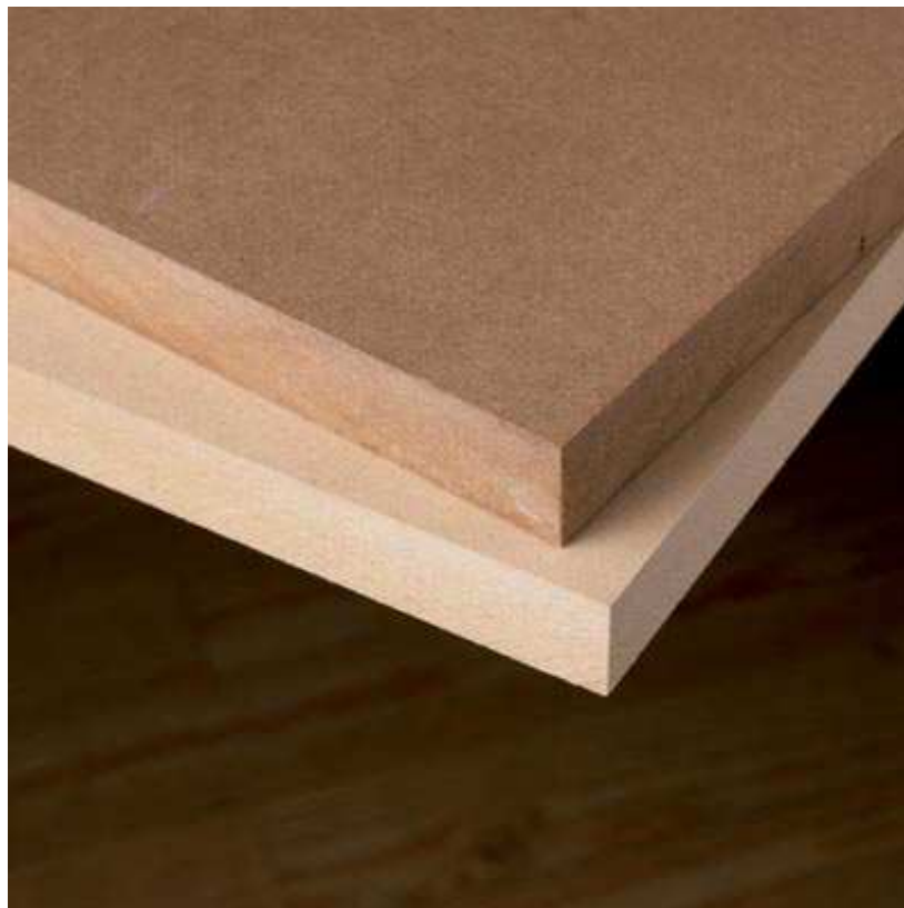
Figura 23. MDF, Medium Density Fiberboard
