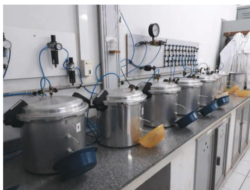
Figura 21 – Aparelho extrator de Richards.
