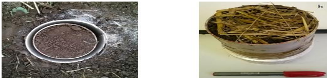
FIGURE 1 Microlysimeter placed into the soil (a) and ML with the equivalent fraction of mulch per treatment (b) showing the seam line sewed upon the ML (b).
