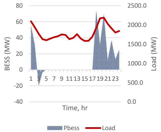
Figure C.20 – Battery Power Injection and Total TSO’s Hourly Load in Area 2: FD Model
