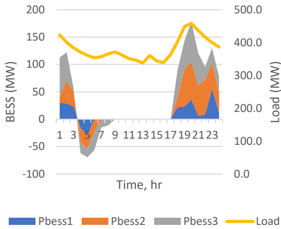
Figure C.6 – Battery Power Injection and Total PAs' Hourly Load in Area 3: FC Model
