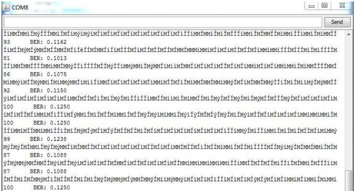
Figura 10 - BER: Rx 1 Led - Tx 1 Led a 40cm
