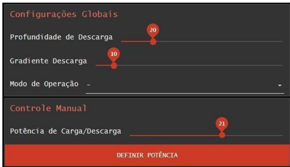
Figura 26 - Dashboard de controle do Inversor via Node-RED
