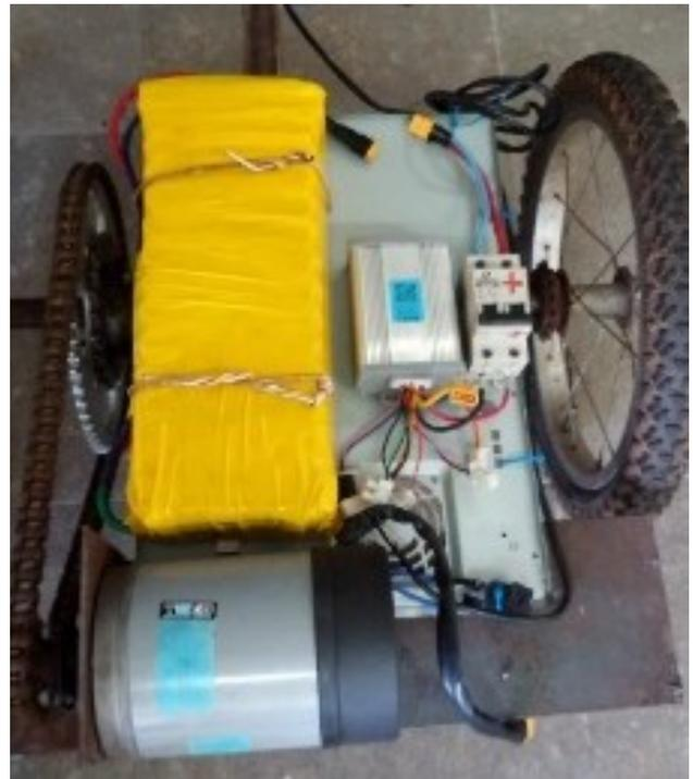
Fig. 3. Bateria, driver e motor.
