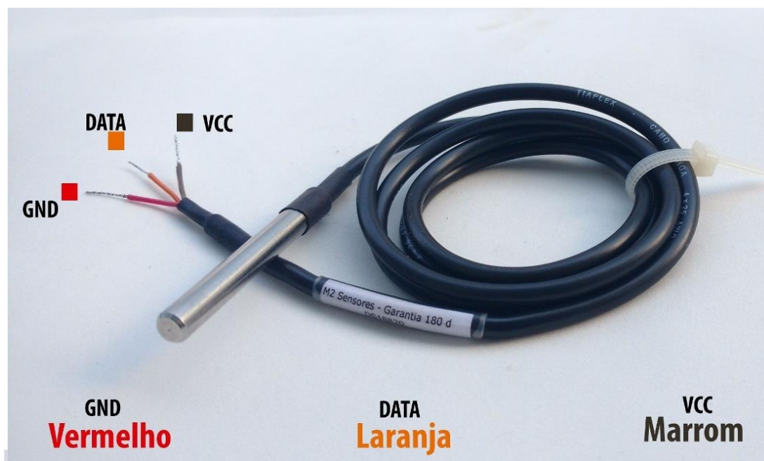
Figura 7 - Sensor DS18B20 (ARDUINOBR,2015)
