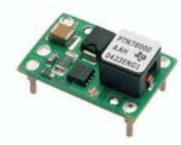
Figura 12 - Conversor CC-CC PTN78000A.
