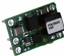
Figura 11 - Conversor CC-CC PTN78000H.
