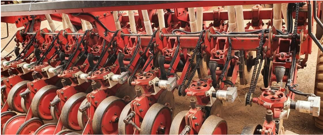
FIGURE 1. Seeder equipped with mechanical transmission and line-to-line electric motors.
