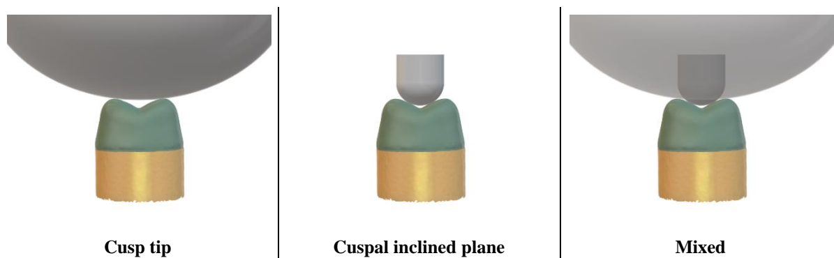
Figure 3. Representations of the region of load application of each experimental group. Load application on the cusp tips was performed with a 40 mm diameter stainless steel load applicator. The load application in the cuspal inclined plane was obtained with a 6 mm diameter stainless steel load applicator, while the mixed group used both load regions and pistons.
