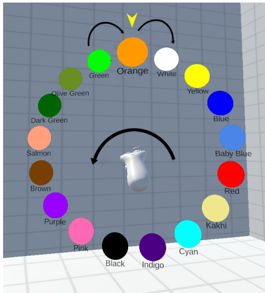
Figure 2: Illustration of how the menu rotates each entry one step in the contrary direction of the wrist rotation
