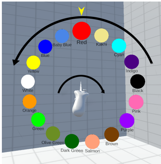
Figure 5: Illustration showing the direction that the menu continuously rotates in the contrary direction that the hand is rotated.
