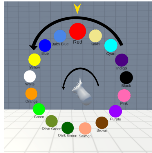
Figure 3: Illustration showing the direction of the rotation of the menu following the rotation of the wrist.
