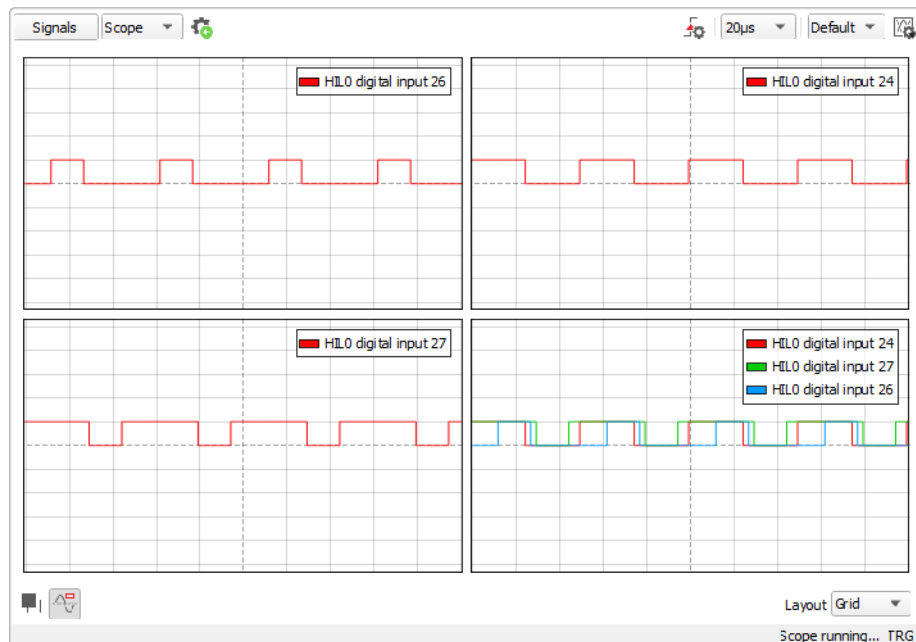
Figura 4.12 – Sinal PWM trifásico - Scope Typhoon
