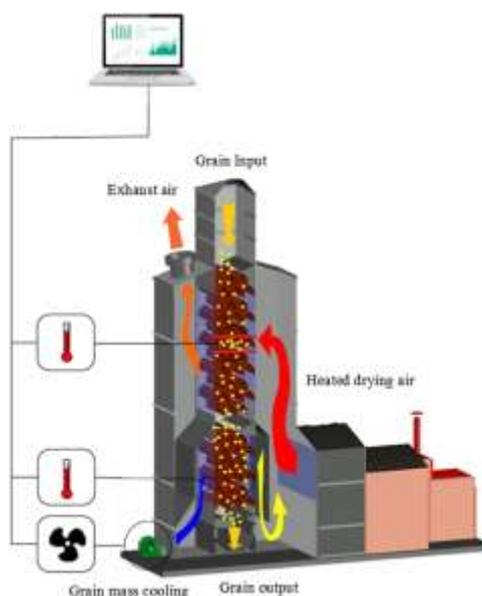
**Fig. 1.** Continuous dryer applied in the soybean drying.
