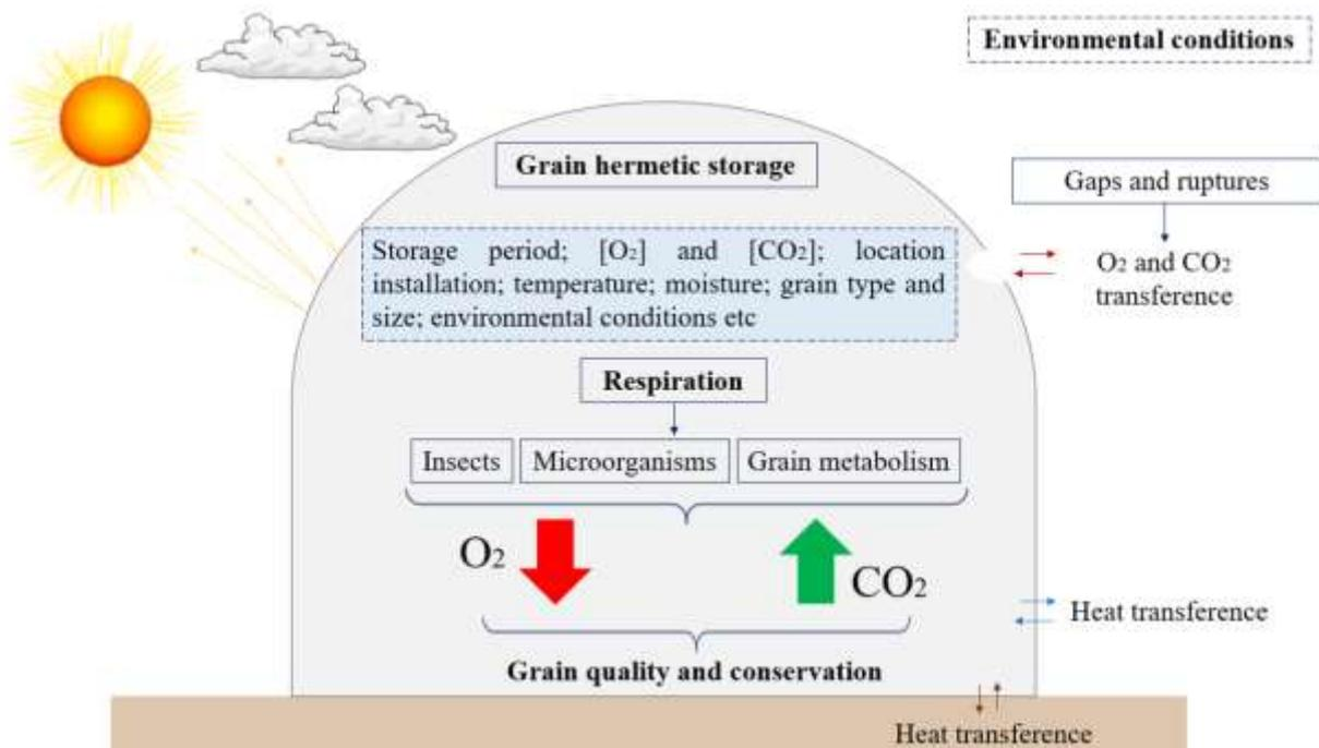
**Figure 6.** Cross section of a bag silo and representation of the factors and processes that are verified in the internal portion of this type of storage.
