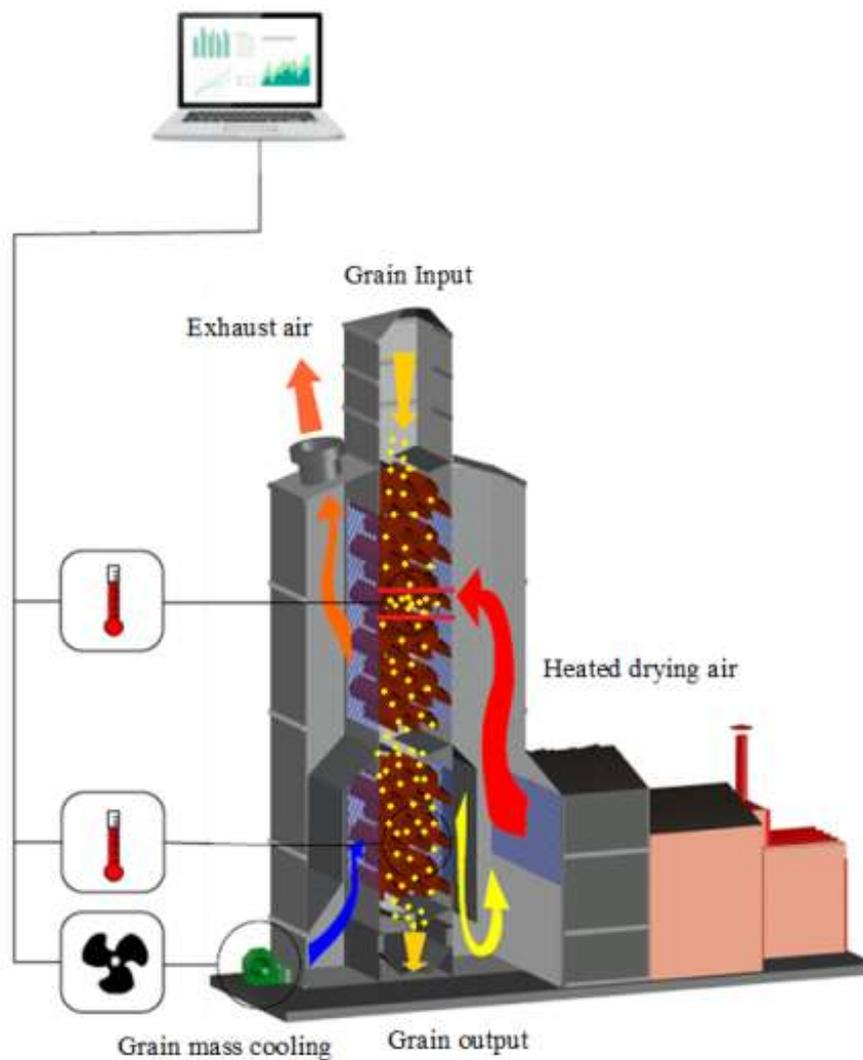
**Figure 1.** Schema of the dryer system.
