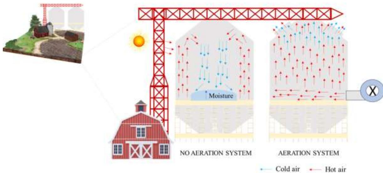
**Figure 7.** Representation of vertical silo and processes that occur in the presence and absence of aeration systems.
