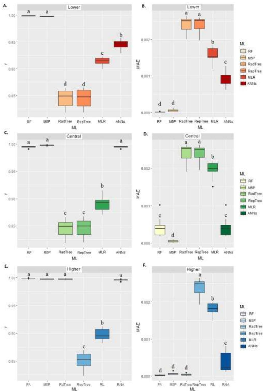
**Fig. 9.** Boxplot for Pearson correlation coefficient ( $r$ ), and mean absolute error (MAE) between observed and estimated values of dry matter loss in soybean grains stored in vertical silo by different machine learning models and inputs. Means followed by equal letters in the same column do not differ by the Scott–Knott test at 5% probability.
