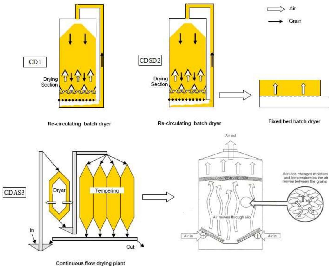
**Figure 4.** CD1 - dry soybeans in continuous dryer, CDSD2 - dry soybeans in continuous dryer + silo-dryer, CDAS3 - dry soybeans in continuous dryer + aerator-silo.
