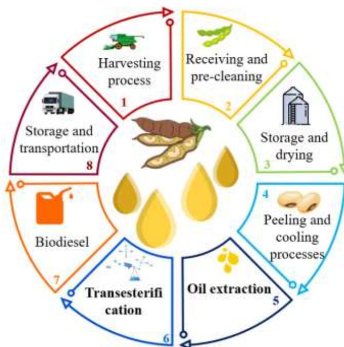
**Figure 8.** Diagram of the main stages of soybean processing to produce biofuels.
