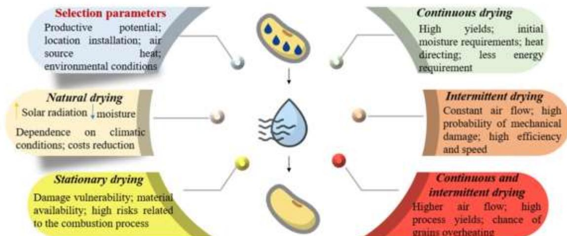
**Figure 2.** Variables considered for the development of the drying stage and the main types of drying applied to soybean grains.
