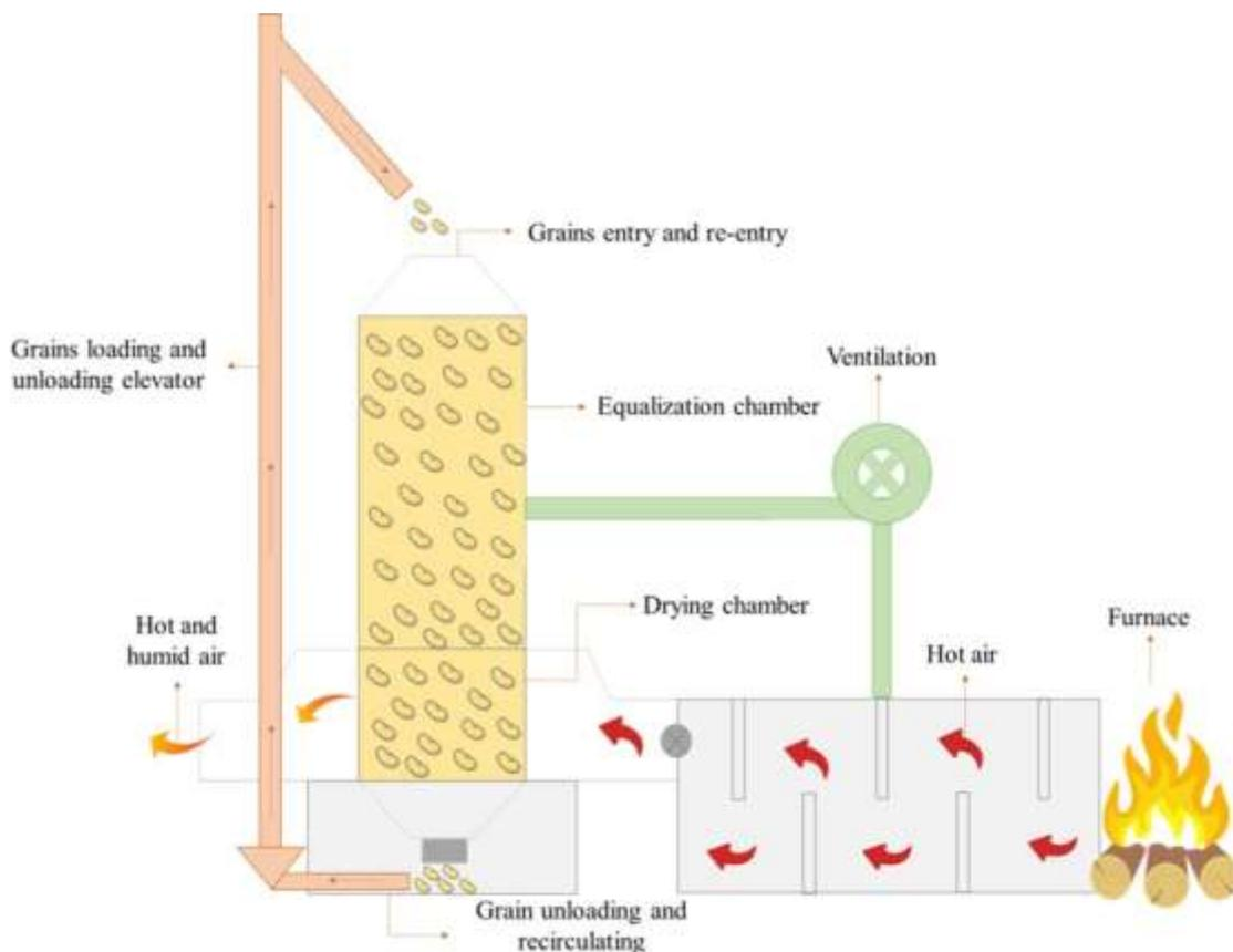
**Figure 4.** Operating dynamics and main flows of the intermittent drying process applied to soybean grains.
