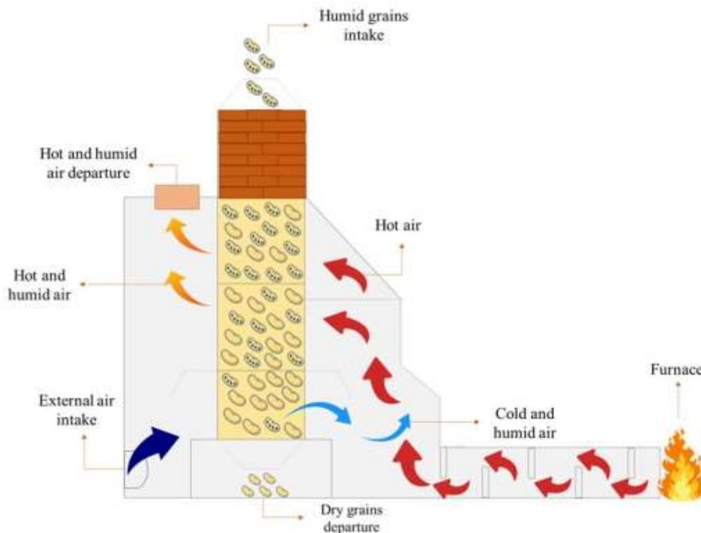
**Figure 3.** Operating dynamics and main flows of the continuous drying process applied to soybean grains.
