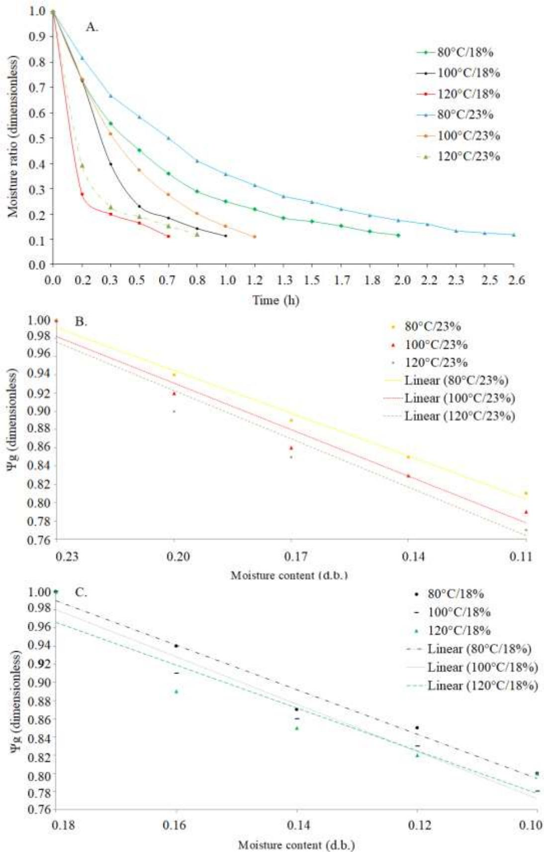
**Figure 2.** Moisture content adjusted by the Wang & Singh model (A), volumetric shrinkage of soybeans in the drying using the model of Rahman, at initial moisture content of 23% (d.b.) (B) and 18% (d.b.) (C).
