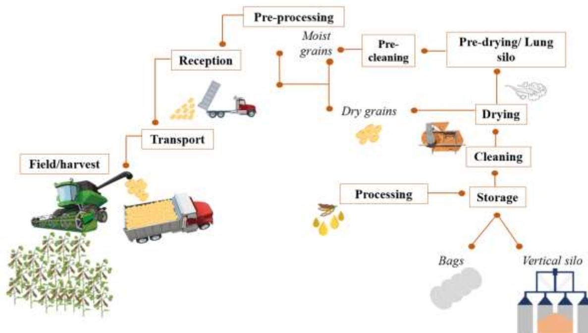
**Figure 1.** Structural diagram of the main processes related to post-harvest during soybean processing.
