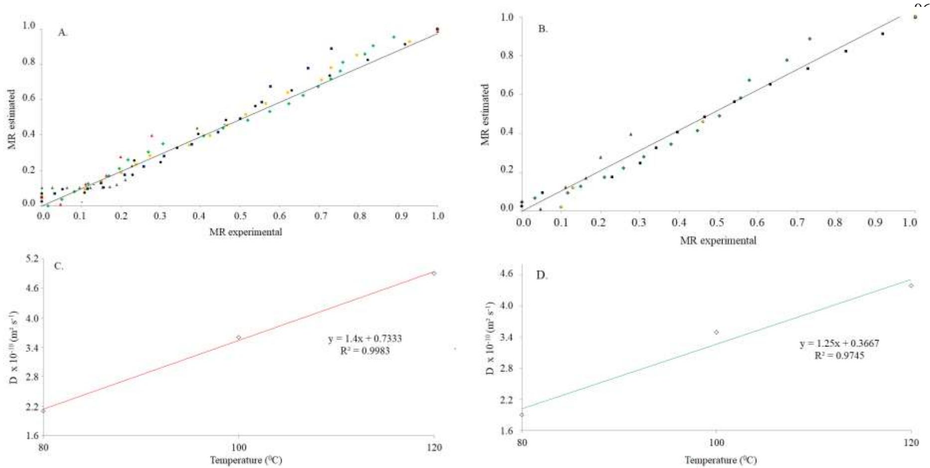
**Figure 3.** Ratio of experimental values and estimated by the Wang & Singh model at initial moisture content of 23% (d.b.) (A); initial moisture content of 18% (d.b.) (B); effective diffusion coefficient ( $\text{m}^2 \text{s}^{-1}$ ) for 23% (d.b.) of the initial moisture content in the grains (C); effective diffusion coefficient ( $\text{m}^2 \text{s}^{-1}$ ) for 18% (d.b.) of the initial moisture content in the grains (D).
