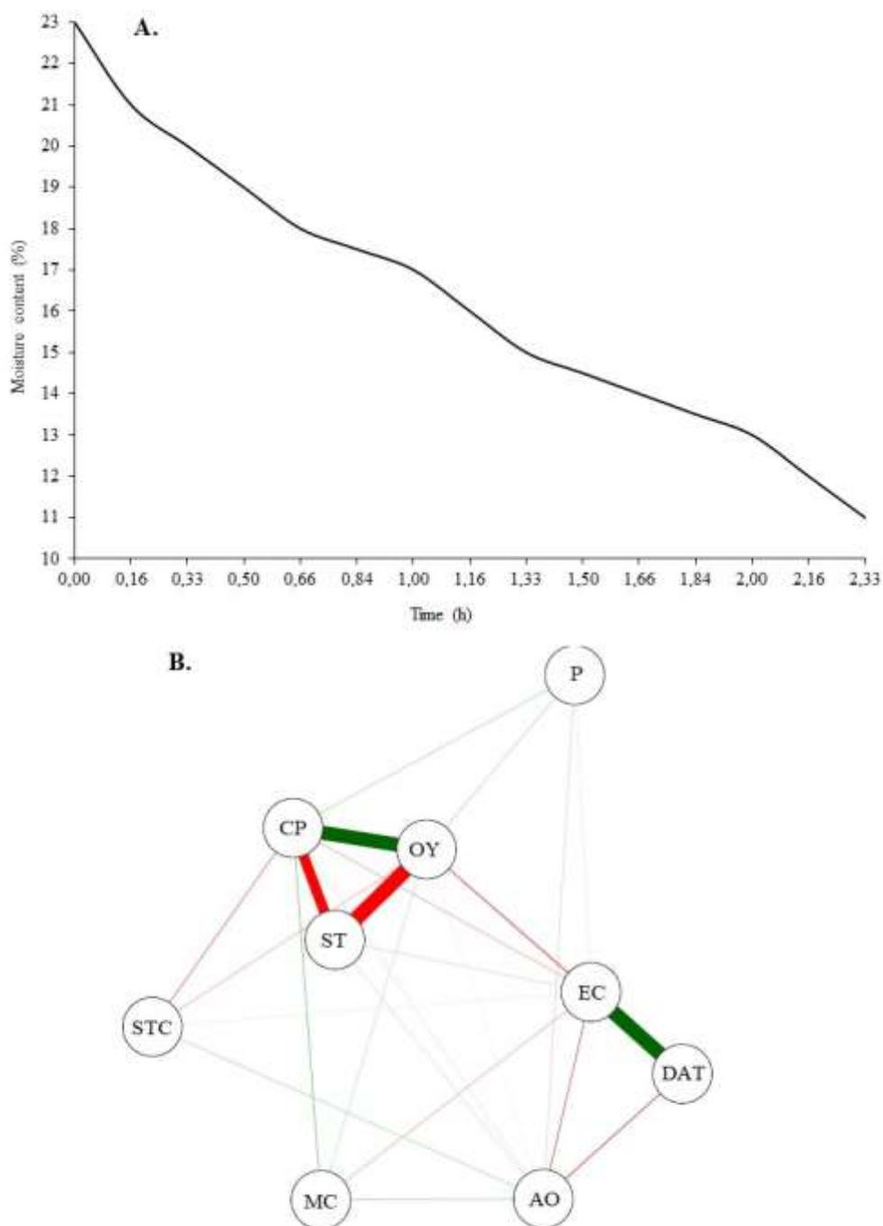
**Fig. 4.** (A) Soybean drying curve, (B) pearson correlation analysis of the qualitative variables (crude protein-CP, acidity oil-AO, oil yield-OY, electrical conductivity-EC, moisture content-IMC, drying air temperature-DAT, packing-P, storage temperature-ST, storage conditions-STC) of soybean grains dry in continuous dryer. Green lines link variables to positive
