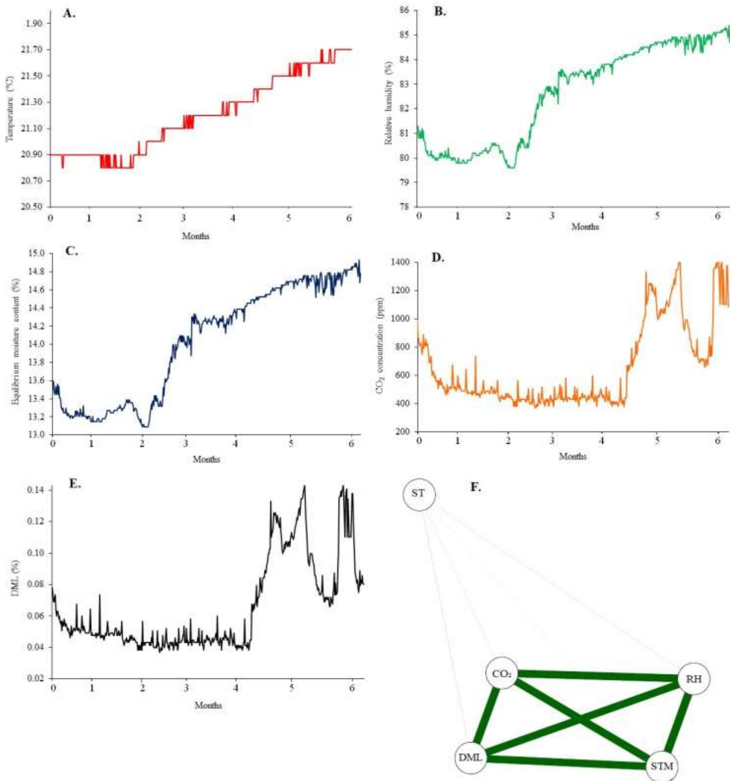
**Fig. 10.** (A) Monitoring of temperature air intergranular, (B) relative humidity air intergranular, (C) equilibrium moisture content, (D) CO<sub>2</sub> concentration, (E) dry matter loss, (F) pearson correlation analysis of the qualitative variables (storage time-STM, storage
