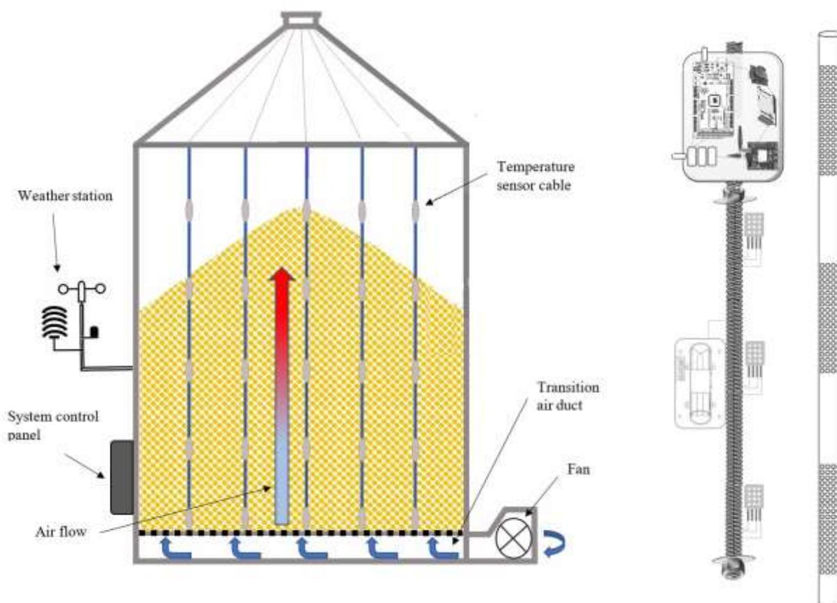
**Fig. 2.** Silo-dryer applied to drying soybeans.
