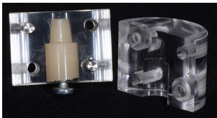
Figure 1. A. Schematic drawing of the composite preparations ( \varnothing : diameter and R: radius) referent to trunked cone. B. Split transparent templates used to produce the composite cores (note the screw on the composite base center).
