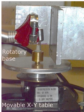
Figure 2. A. Special device for grinding the composite preparations. B. Composite core after grinding (bur positioned parallel to the composite surface). C. Micrometer installed onto a movable X-Y table to standardize the grinding pressure.
