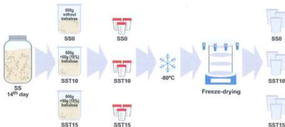
Fig. 2. Process of freeze-drying of "spontaneous" sourdough (SS). SS0: "spontaneous" sourdough without trehalose; SST10: "spontaneous" sourdough with 10% trehalose; SST15: "spontaneous" sourdough with 15% trehalose.
