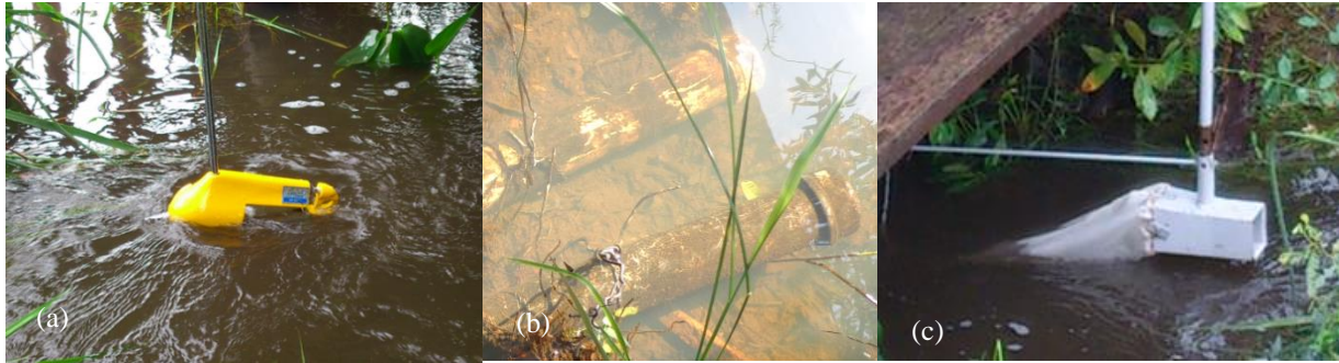
US-DH-48 type sampler used for the sampling of suspended sediments (a), time-integrating suspended sediment samplers (b) and US-BLH-84 sampler for the collection of transported sediments in drag (c) (Photos: Author).
