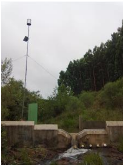
Automated hydro-sedimentometric monitoring sections in the catchment with eucalyptus (a) and with grassland (b) in São Gabriel-RS.
