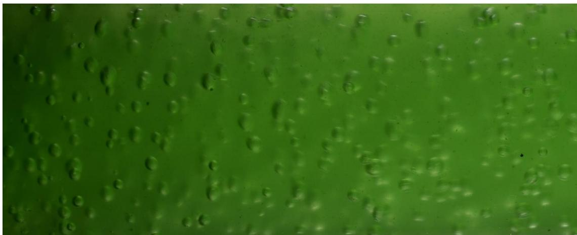
Fig. 1 Example of the obtained photograph by ozone-flotation to determine bubble size.
