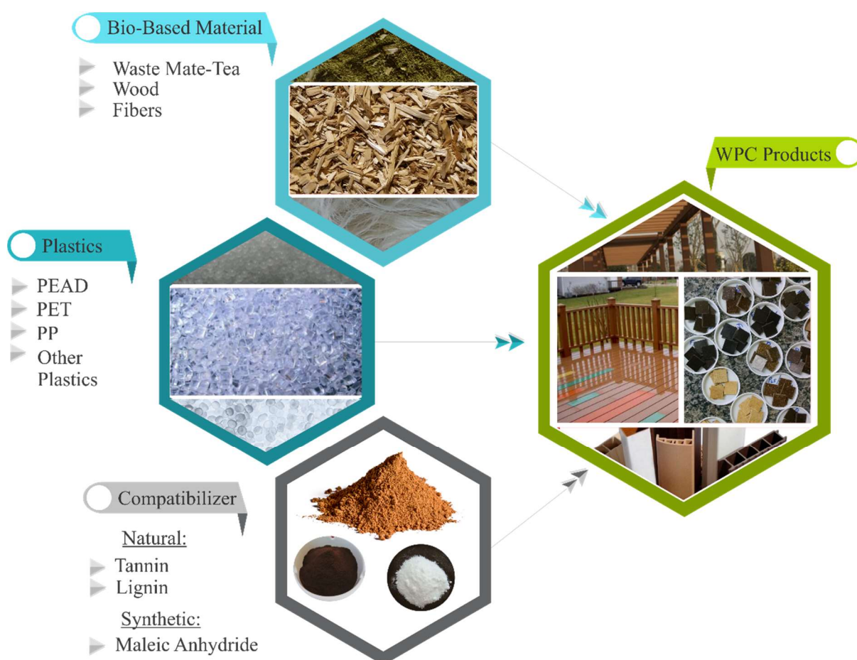
Figure 4. Examples of raw material components in WPC products
