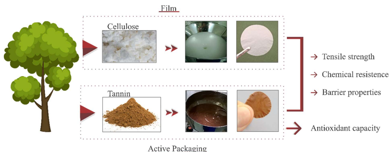
Figure 5. Films formed from nanocellulose and tannin.
