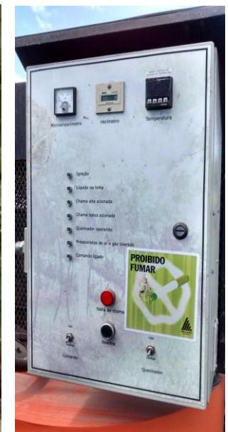
**Figure 1** Thermal Pest Control equipment used for grape treatment. A) Lateral overview of the equipment being towed by a tractor. B) Back view of the equipment. C) Control monitor for Thermal Pest Control treatment conditions.
