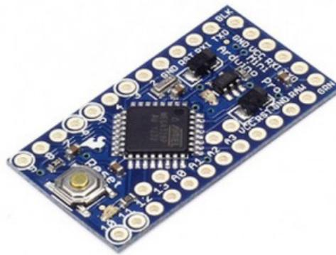
Figura 2.4 – Arduino Pro Mini
