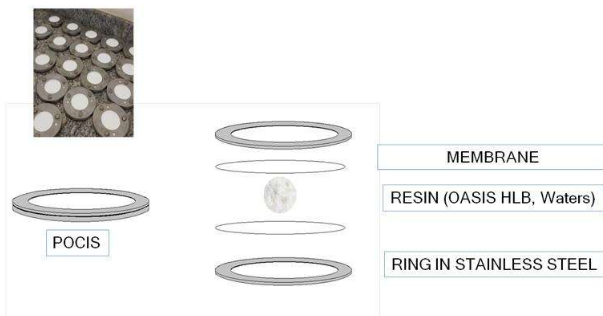
Chapter 2 - Figure 27 – POCIS sampling method
