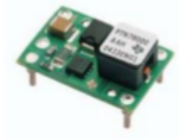
Figura 25 - Conversor CC-CC PTN78000A [TEXAS INSTRUMENTS, 2006].
