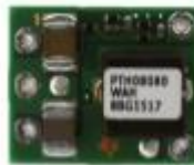
Figura 26 - Conversor CC-CC PTH08080W [TEXAS INSTRUMENTS, 2013].
