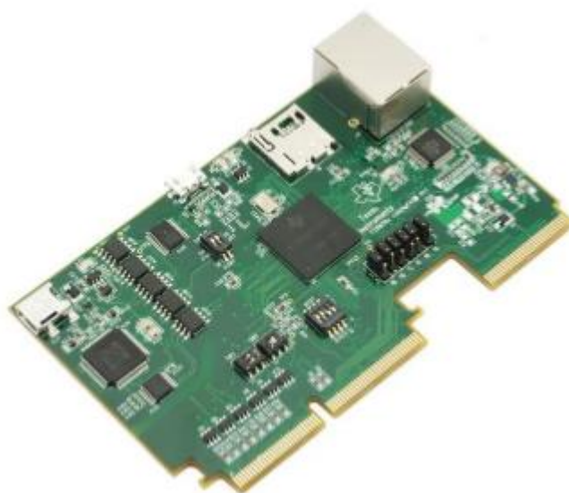
Figura 30 - Microcontrolador Converteo F28M36x [TEXAS INSTRUMENTS ,2016].
