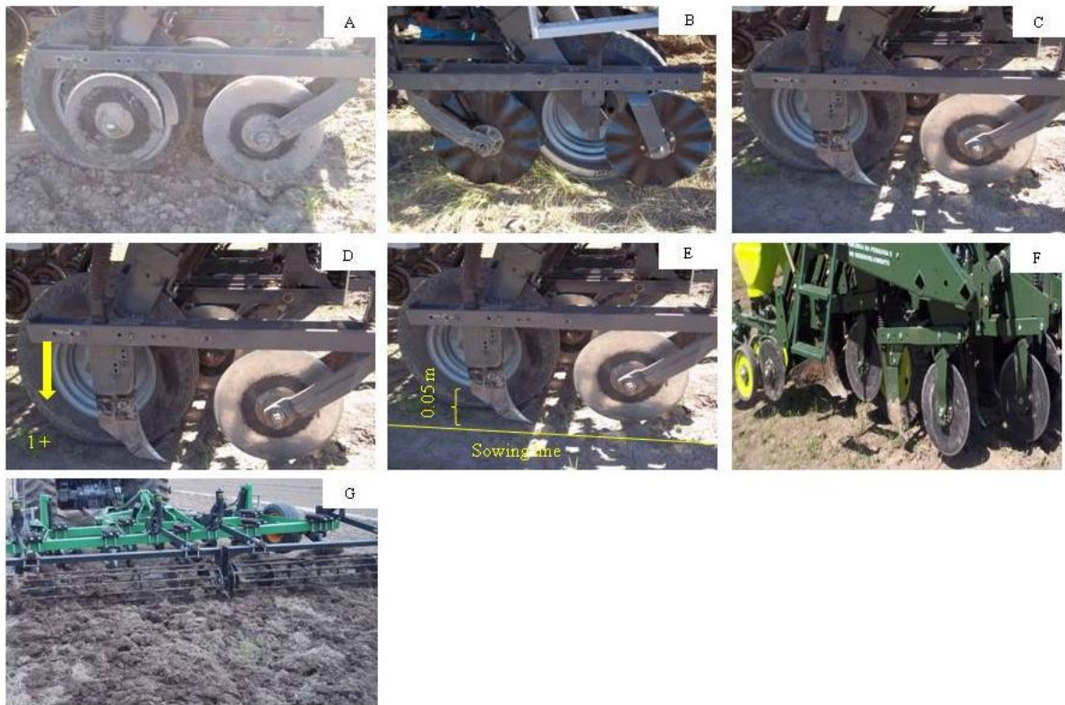
Figure 2. Tillage systems used for soybean: sowing with offset double disc (a); sowing with a fluted coulter disc (b); sowing with a knife runner opener (c); sowing with a knife runner opener + press wheel mechanism for ground levelling (1) (d); sowing with knife 0.05 m from the planting row (e); raised bed system (f); and chisel plough + sowing using a offset double disc (g). Santa Maria, Brazil. Arrow indicates position in which the soil press wheel mechanism for ground levelling was placed.
